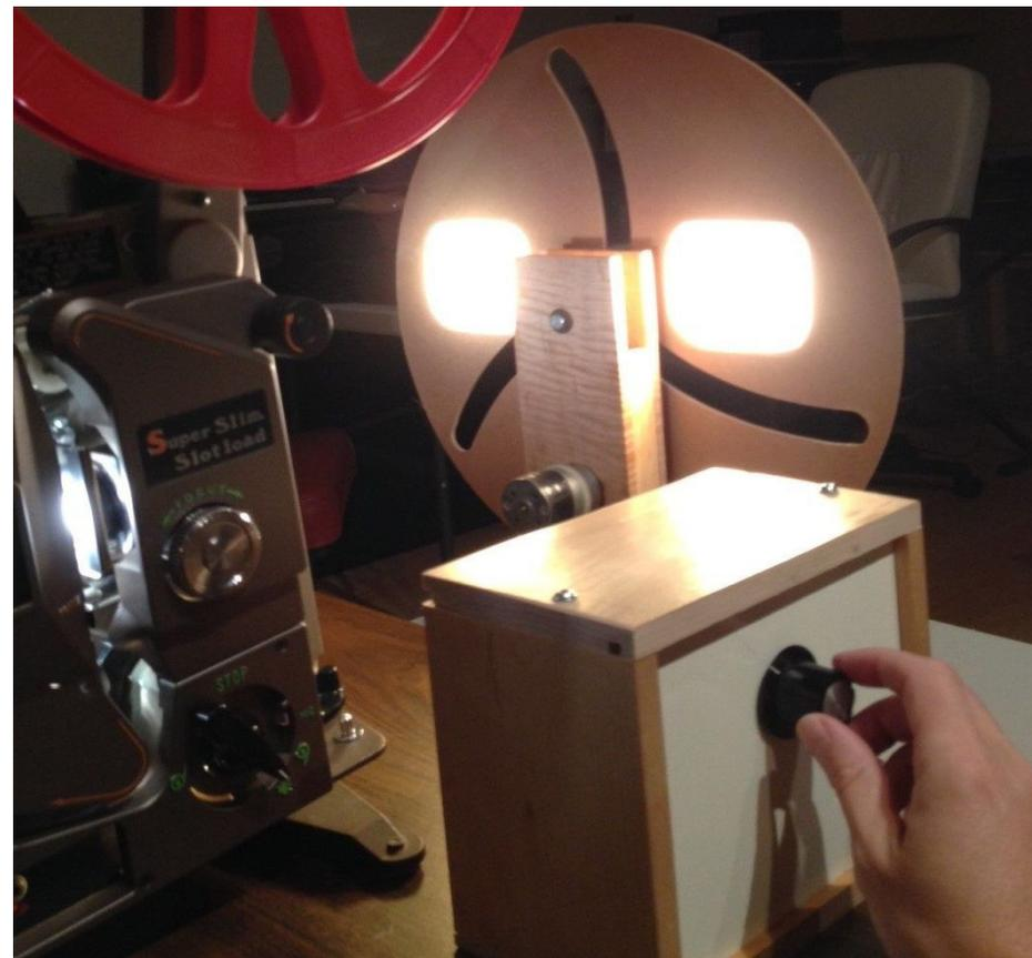
Figure 2: Variable-speed rotating shutter disc used in *The Velvet Underground* event.
