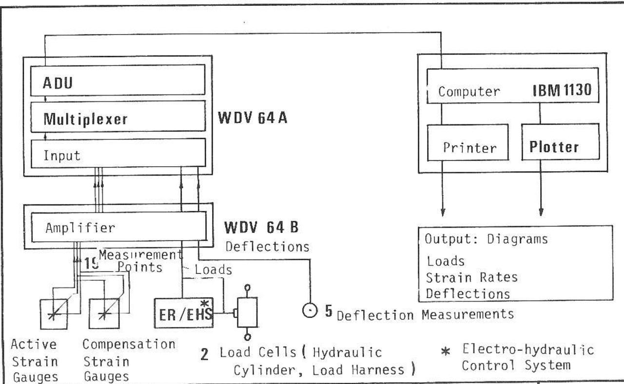
**DFVLR** Block Diagram of Data Acquisition and Reduction for Static Tests on CFRP Wing Fig. 9
