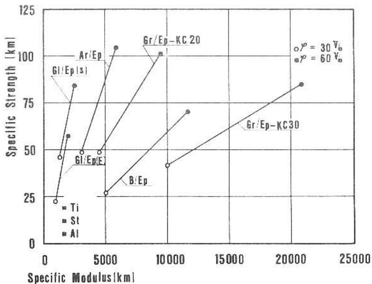
Fig.1 Specific Strength vs. Specific Modulus UD-Composites, Ref. [1]
