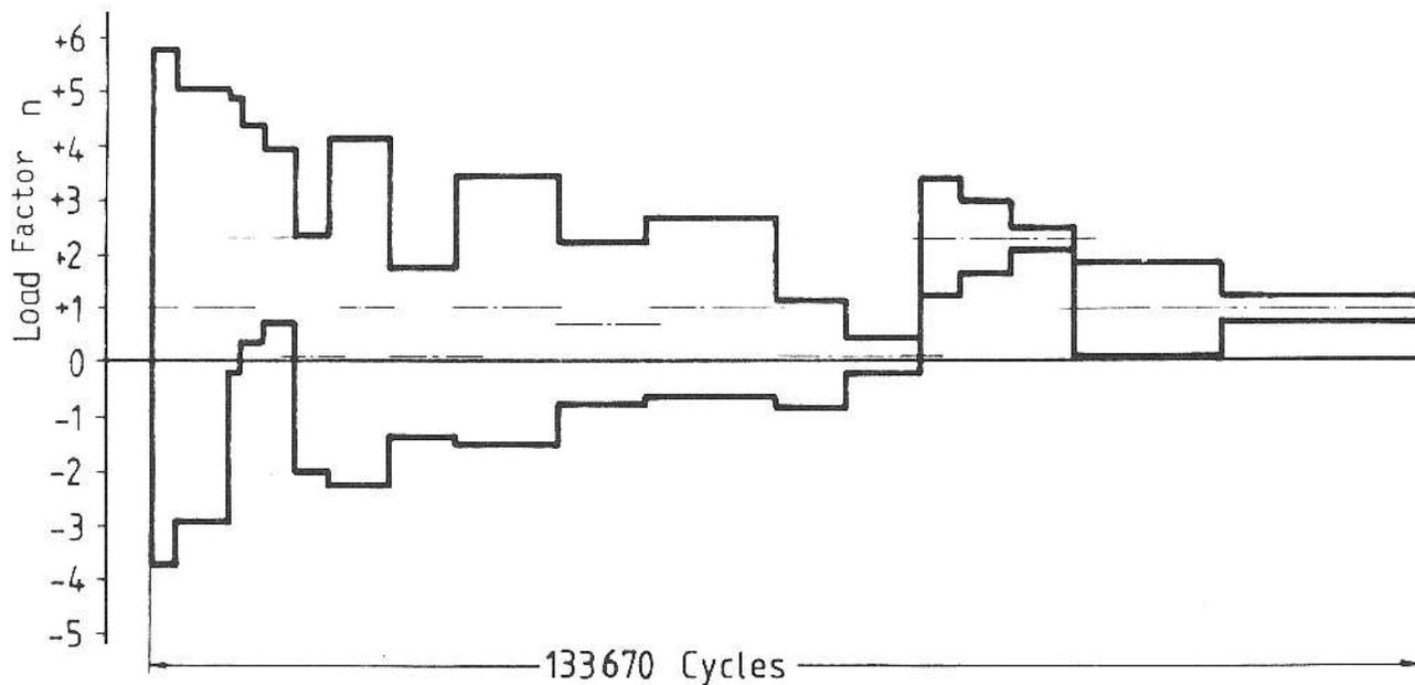
Fig.11 Splitting and Rearrangement of the Service Life Program for 24h - Cycle
