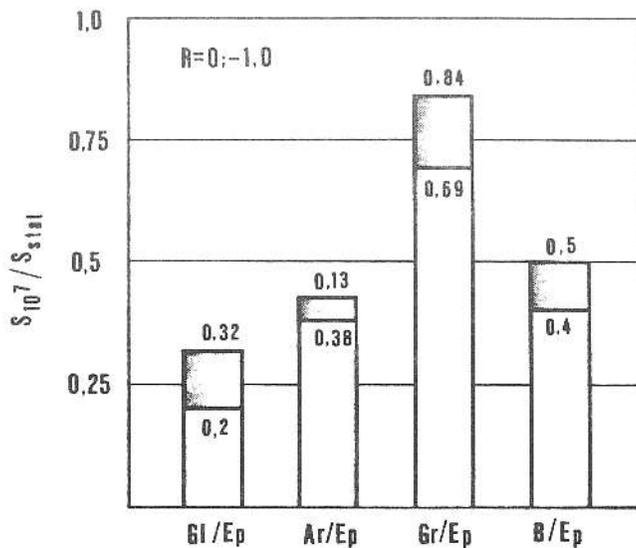
Fig.2 Fatigue limits of UD composites [4]
