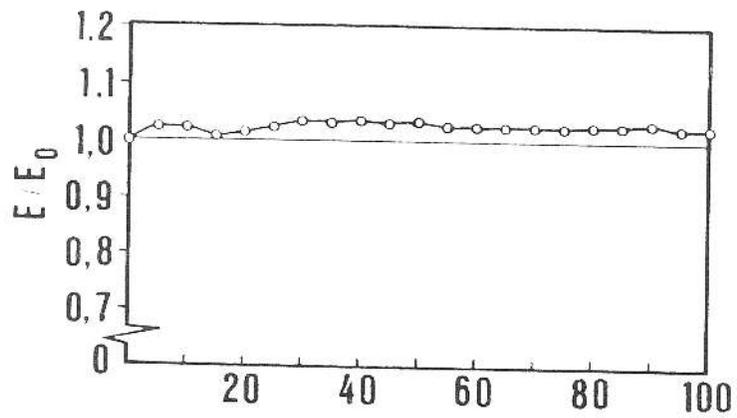
Fig. 15: Variation of Relative Stiffness of the CFRP Wing
