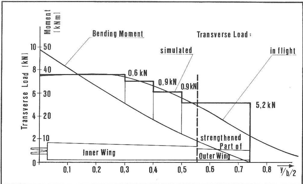
**DFVLR** Simulated Transverse-Load Distribution, Resulting Bendingmoment Fig. 8
