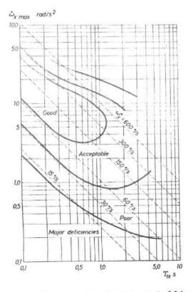
Fig. 10 Pilot Opinion on Rolling Mode (after O'Hara(31})
