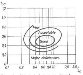
Fig. 6 Pilot Opinion on Short Period Frequency and Damping (after O'Hara(33)resp. Shomber & Gertsen<sup>(32)</sup>)
