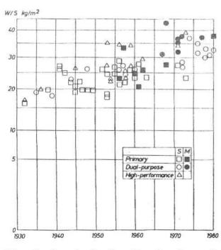
Fig. 3 Trends in the Wing Loading of Two-Seaters
