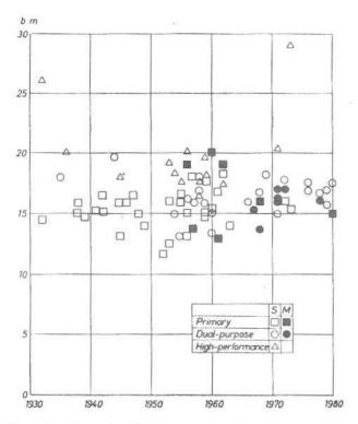
Fig. 1 Trends in the Span of Two-Seaters (S=Sailplane, M=Motorglider)
