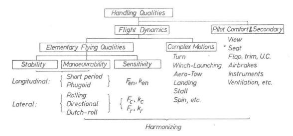
Fig. 5 Classification of Handling Quality Requirements
