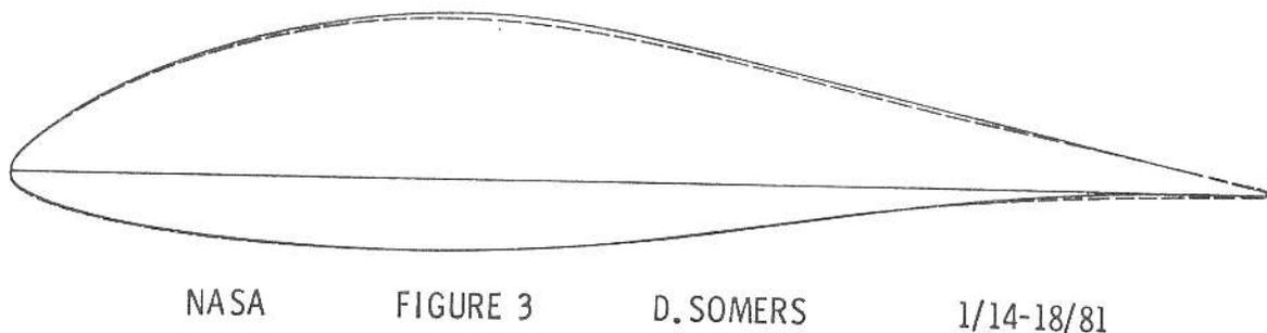
considerable differences are apparent. Obviously, these differences cannot be corrected by sanding alone. The results from this wind-tunnel test are given in NASA TN D-8324 entitled "Experimental and Theoretical Low-Speed Aerodynamic Characteristics of a Wortmann Airfoil as Manufactured on a Fiberglass Sailplane" by Dan M. Somers.
