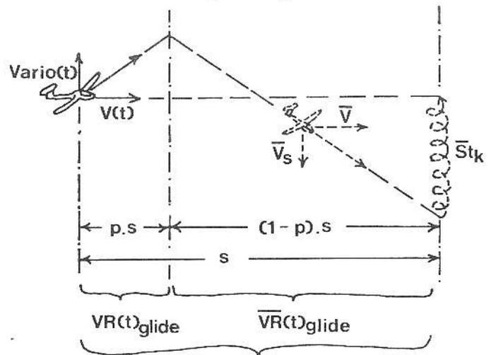
$$VR^+(t)_{\text{glide}} = \frac{1}{\frac{p}{VR(t)_{\text{glide}}} + \frac{(1-p)}{\overline{VR}(t)_{\text{glide}}}}$$
