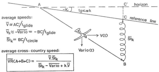
$$\overline{VR}_{ABC} = \frac{S_{AC}}{t_{AB} + t_{BC}} = \frac{\overline{St}_{k} \cdot \overline{V}}{\overline{Vs} + \overline{St}_{k} + k \cdot \overline{V}}$$
