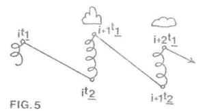
it] t it2; (i = number of section; l = pilot stops thermaling and starts interthermal cruise; 2 = pilot stops interthermal cruise and starts thermaling in the updraft)
