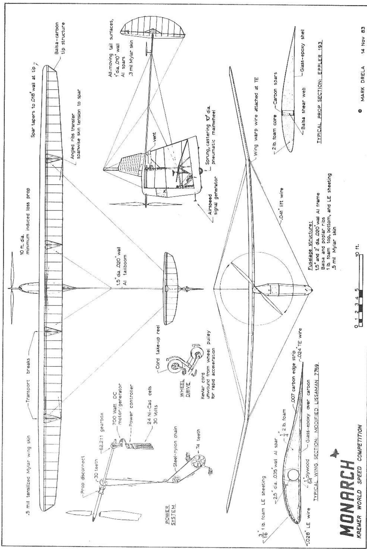
FIGURE 1. the MIT Monarch Human-Powered Aircraft. September 1983 Flight Version.
