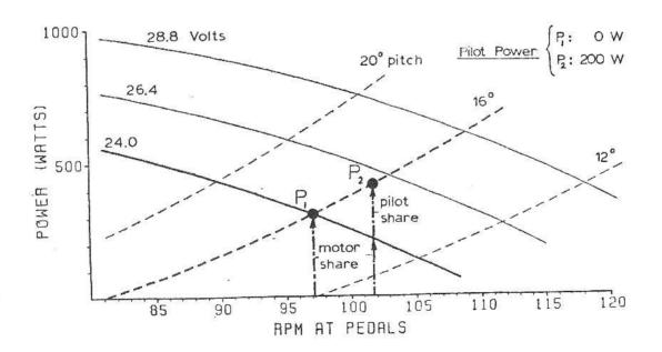
Figure 2. Operating curves for motor (solid line)and propeller (dashed) at various voltage and pitch settings at a flight speed of 23 mph.
