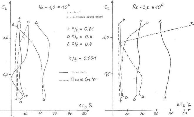
Figure 11: Alteration of drag by a trip wire on the upper airfoil surface
