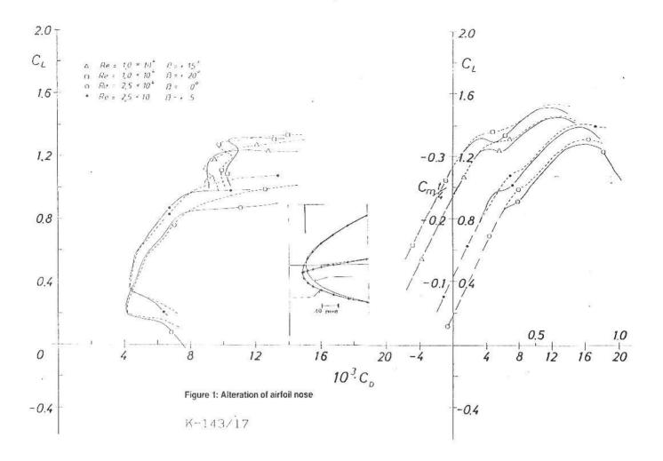
the increase of drag on the upper range of the laminar bucket is less. This is to be expressed in the  $c_a(\infty)$ -curve. The stall characteristics are somewhat more favorable. Figure 2 shows comparative measurements of another airfoil with flaps. Here, above all, the maximum lift and the stall characteristics are improved.
