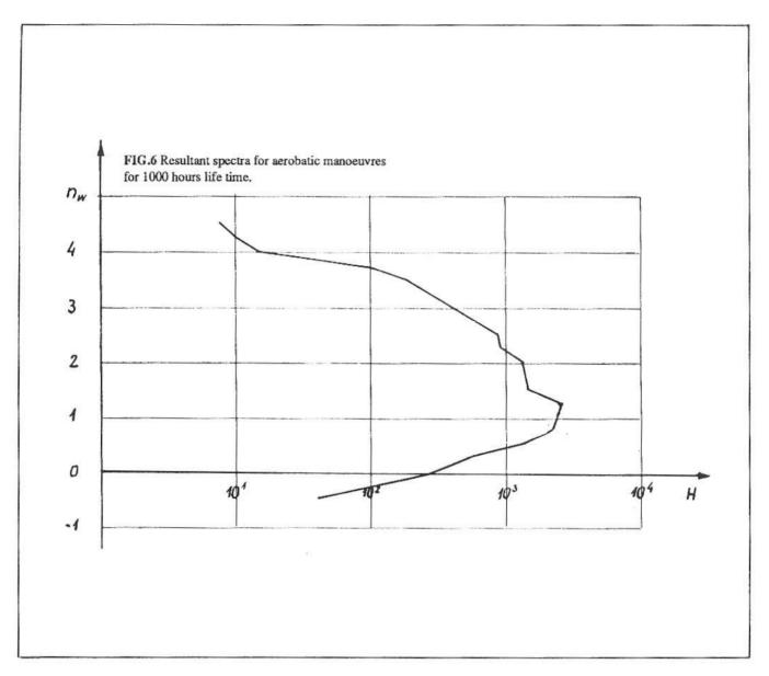
(Table II). The cycles defined for 100 manoeuvres ( $H_{100}$ ) should be multiplied by the factor:  $k_{\rm LT} = F_{\rm LT}/100$  to obtain the total 1000 hours life time cycles for every manoeuvre. (For  $F_{\rm LT}$  values see table II.) The sum of:  $H_{\rm LT} = k_{\rm LT} \cdot H_{100}$  for all the manoeuvres gives the resultant cycle amount for the 1000 hours spectrum (H).
