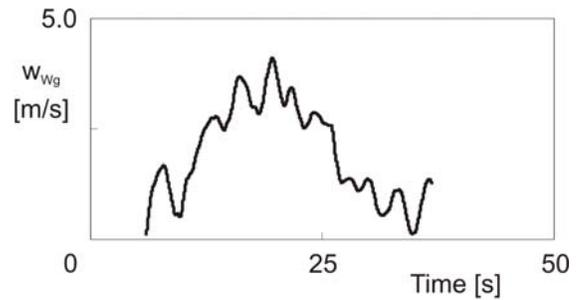
**Figure 10** Vertical wind speed component during a test flight through a thermal.
