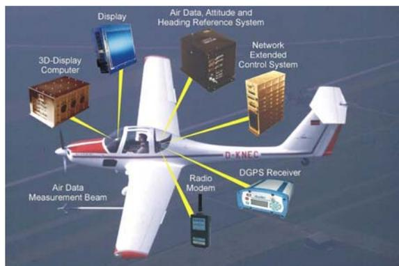
**Figure 5** Research aircraft with test equipment
