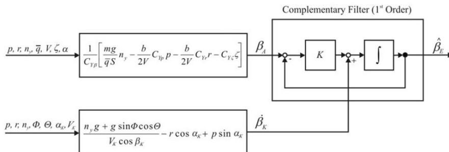
**Figure 4** Module for angle of sideslip determination
