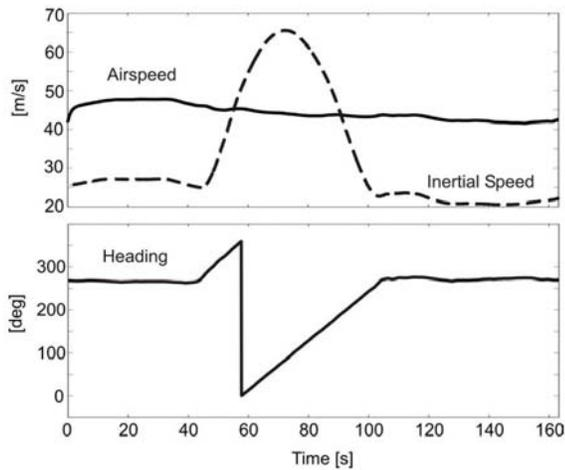
**Figure 8** Speeds and heading during a turn in a constant wind field.
