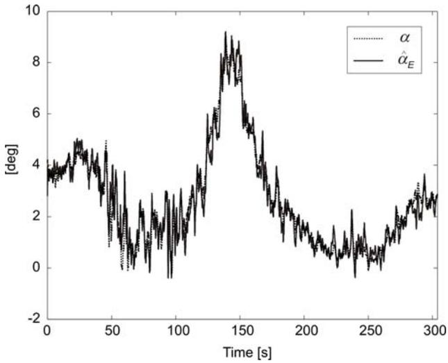
**Figure 7** Results from flight tests for angle of attack determination.
