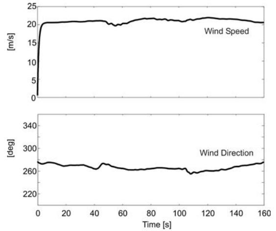
**Figure 9** Wind speed and direction during a turn in a constant wind field.
