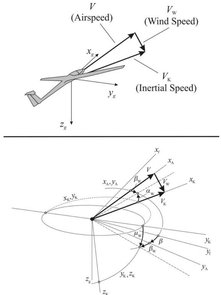
Figure 1 Speed vectors and coordinate systems
