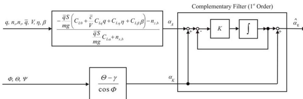
**Figure 3** Module for angle of attack determination
