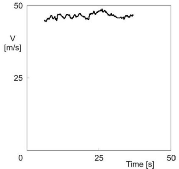
**Figure 11** Airspeed during a test flight through a thermal.
