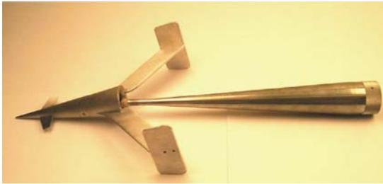
**Figure 6** Aerodynamic sensor for angles of attack and sideslip and for true airspeed.
