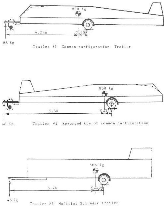
FIGURE 3. Schematics of glider trailers used in this study.
