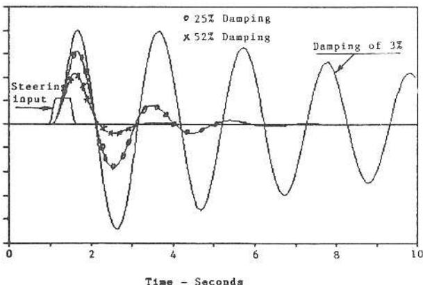
FIGURE 2. Various damped articulation responses to steering input.
