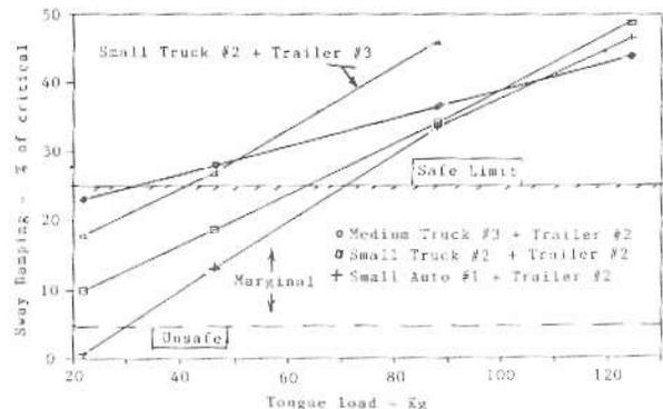
FIGURE 7. Sway damping of trailer #2 towed at 100 km/hr.
