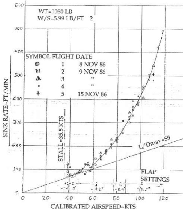
sufficiently tested the Reference B wing relative profile drag probe to have fairly good confidence in its ability to indicate near optimum flap settings for our flight test polar measurements. Therefore, that instrument was installed during all recent flight tests and used to determine the best flap setting at each airspeed. Those flap angles are noted on the lower portion of Figure 4.
