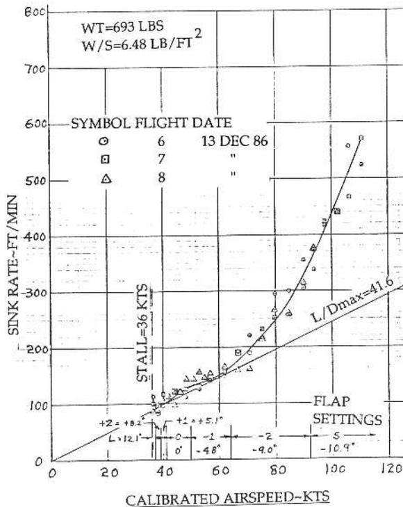
When the Ventus A was initially tested in 1981, it was in its 15 meter wingspan configuration (Reference D). At that time sink rate tests were performed both with and without the factory supplied dimpled turbulator strips installed at .80c. Better performance was measured without the turbulators installed, so they were then removed for the following 15 meter and 16.6 meter wingspan testing; where excellent  $L/D_{max}$  values of about 45 and 50, respectively, were measured.
