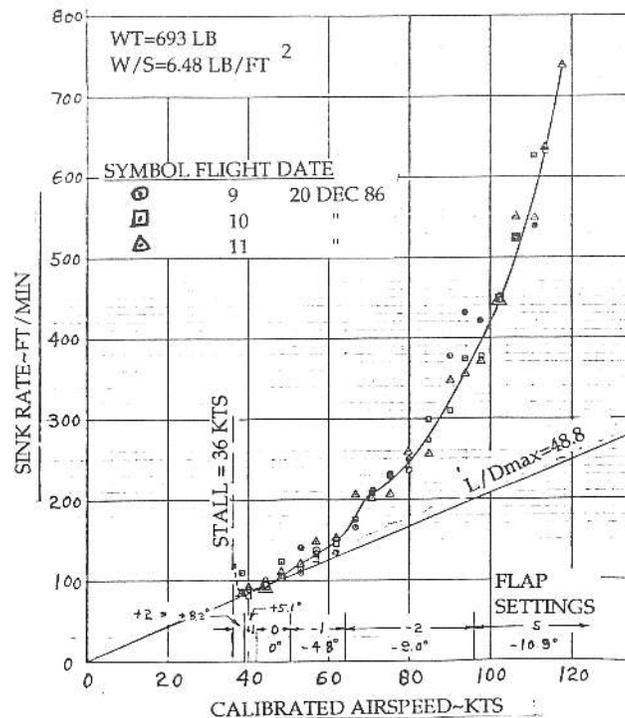
below 65 kts. An  $L/D_{max}$  of about 48.8 was shown at 44 kts, with equal or slightly better sink rates measured at airspeeds above 70 kts. This unexpectedly large performance improvement to the Ventus' polar is puzzling, especially since the recent Nimbus 3 testing with the same airfoil had shown excellent performance with the turbulators installed.
