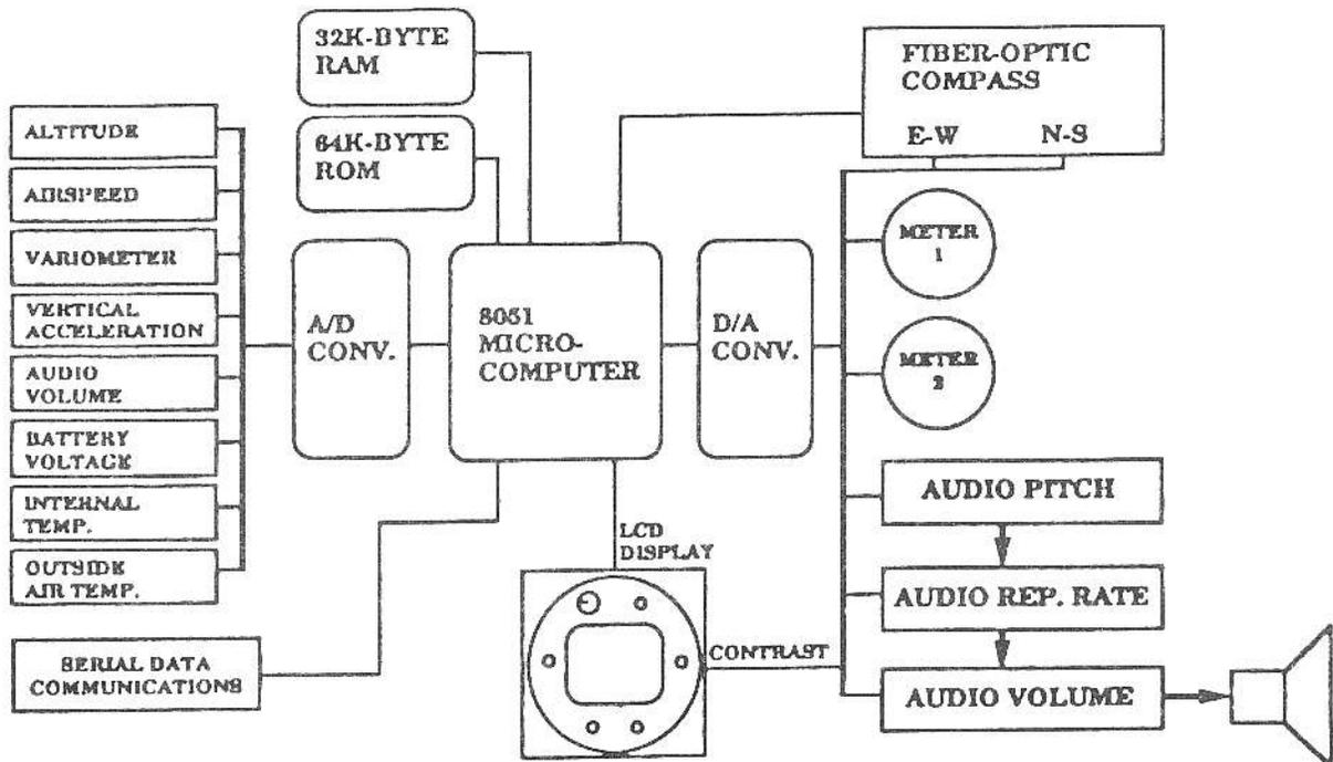
Figure 7. Block diagram of the S-NAV.
