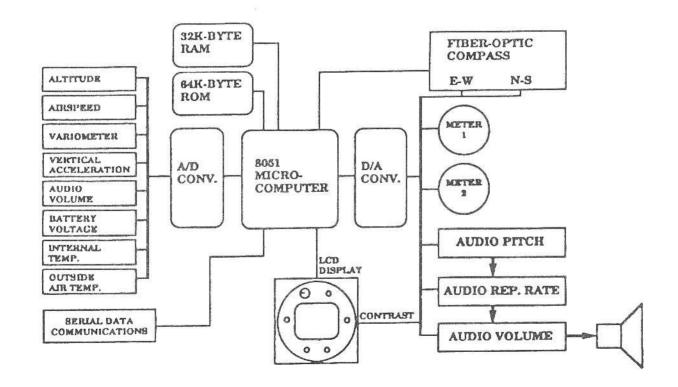
Figure 7. Block diagram of the S-NAV.
