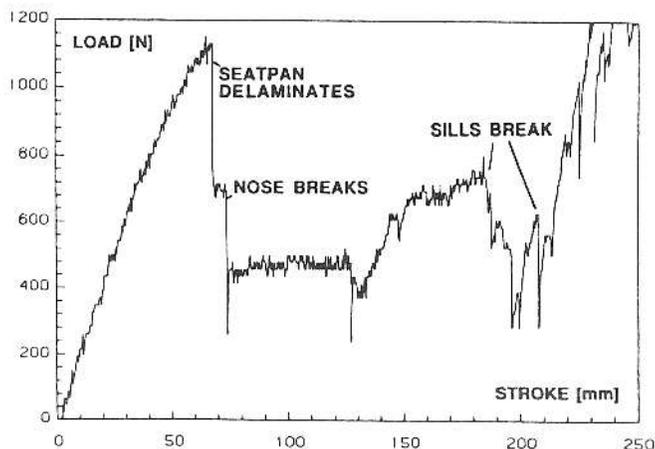
Figure 5. Load vs. stroke for the E-glass fuselage.
