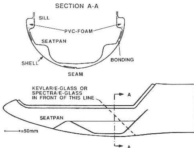
Figure 4. Geometry of the test fuselage articles.
