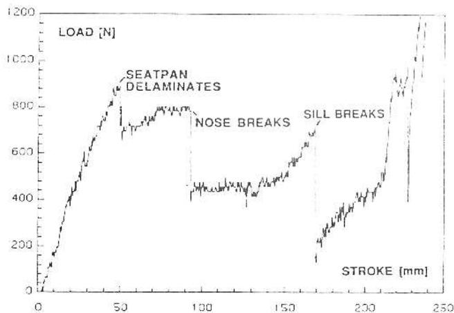
Figure 6. Load vs. stroke for the Kevlar/E-glass fuselage
