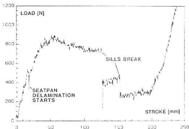
Figure 7. Load vs. stroke for the Spectra/E-glass fuselage
