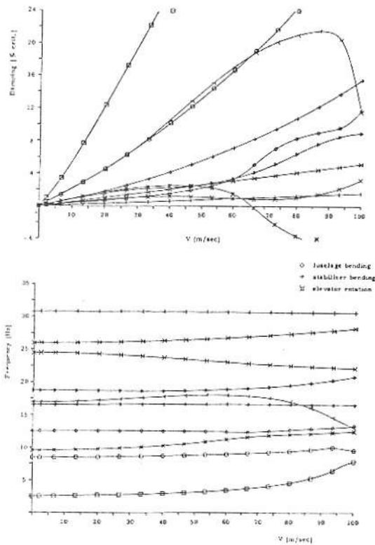
FIGURE 11. Symmetrical flutter calculation (glider B).
