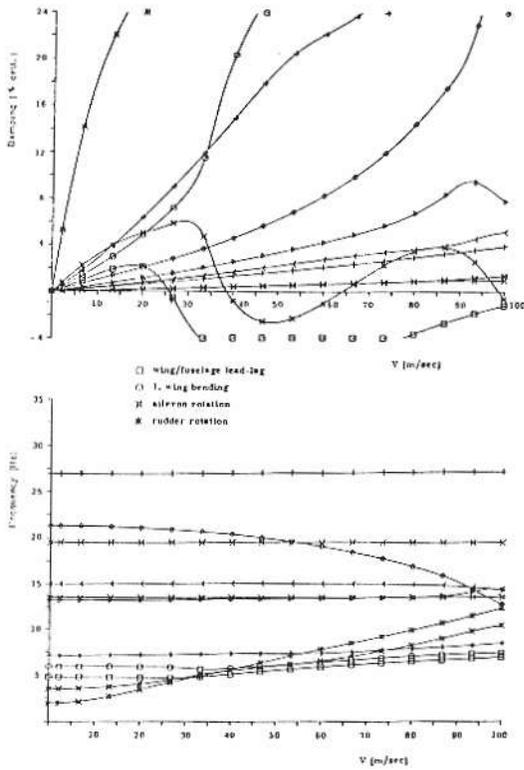
FIGURE 10. Antisymmetrical flutter calculation (glider B).
