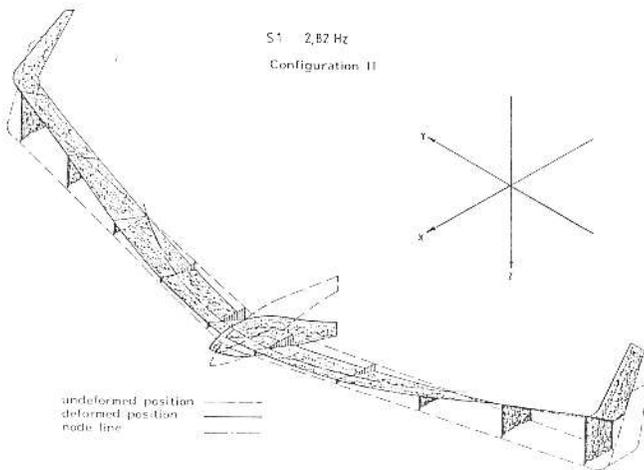
FIGURE 14. Fundamental bending mode of tailless SB-13 glider model.
