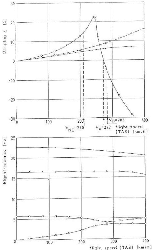
FIGURE 17. Flutter calculation of SB-13 final design.
