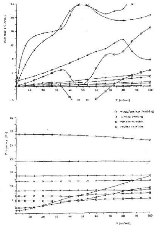
FIGURE 12. Antisymmetrical flutter calculation (glider C).
