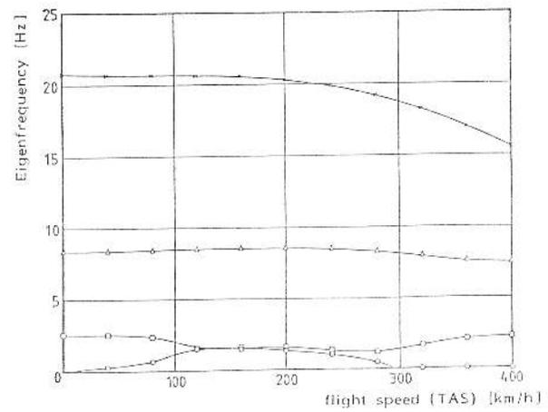
FIGURE 15. Flutter calculation of SB-13 preliminary design.
