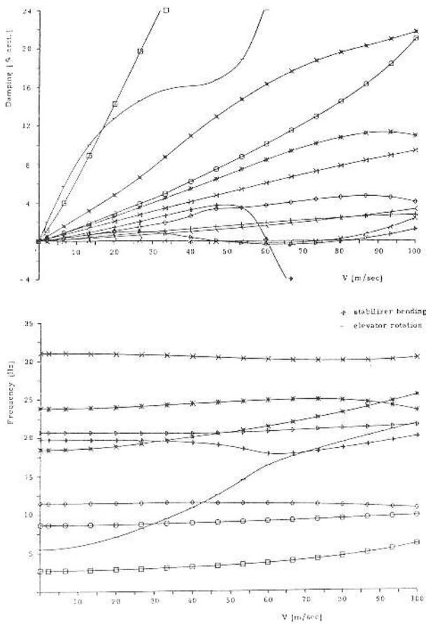
FIGURE 13. Symmetrical flutter calculation (glider D).
