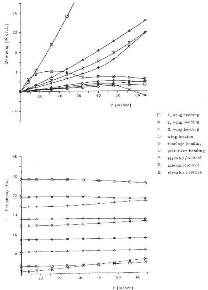
FIGURE 6. Symmetrical flutter calculation (original glider A).
