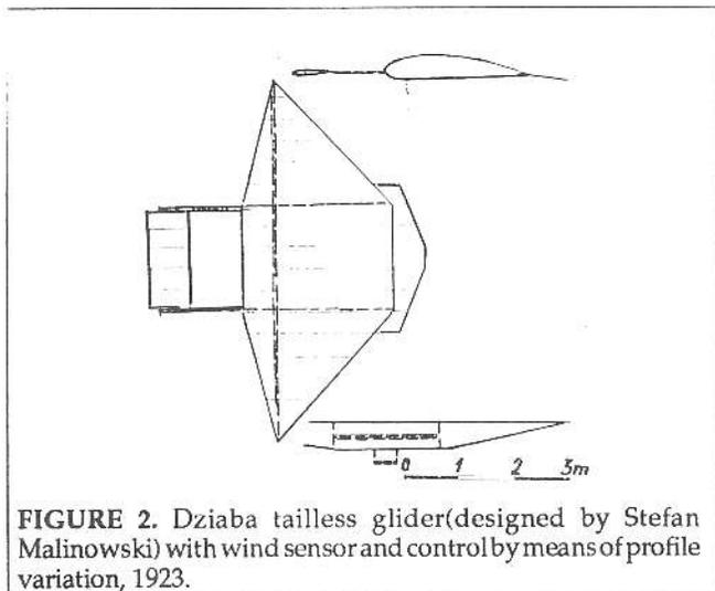
FIGURE 2. Dziaba tailless glider (designed by Stefan Malinowski) with wind sensor and control by means of profile variation, 1923.
