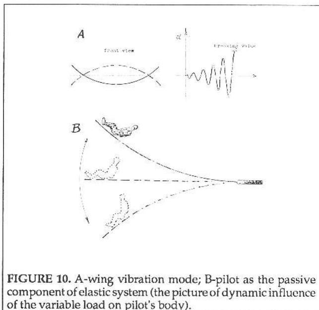
FIGURE 10. A-wing vibration mode; B-pilot as the passive component of elastic system (the picture of dynamic influence of the variable load on pilot's body).
