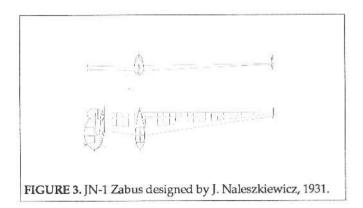
The first flight was made in June 1932 at Deblin airfield by Captain Franciszek Jach. Bungee take off was used initially, then motor car tows. The results were, however, not satisfactory. Too high elevator sensitivity and violent stalling led to serious damage that stopped further testing.
