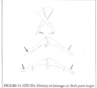
to rotate one onto another; b). Left wing root end destroys the canopy; c). Further collision of both parts of the wreckage.
