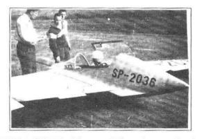
PHOTO 2. SZD-20x. Elevator deflected upwards when stick is pushed forwards!
