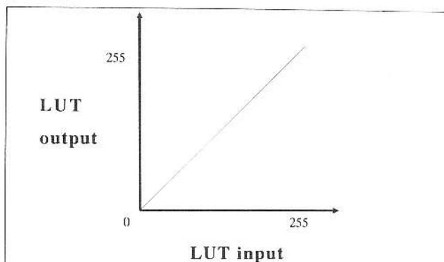
FIGURE 3 (a). LUT transfer function for positive camera image.
