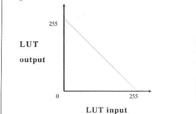
FIGURE 3 (b). LUT transfer function for negative camera image.
