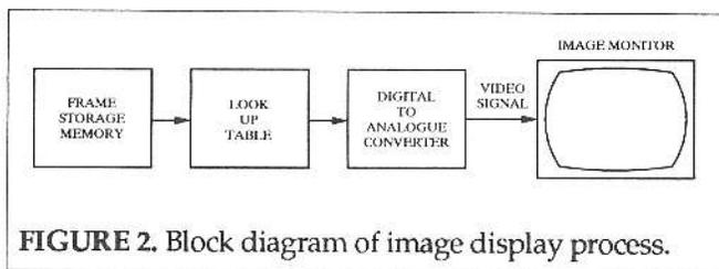
FIGURE 2. Block diagram of image display process.
