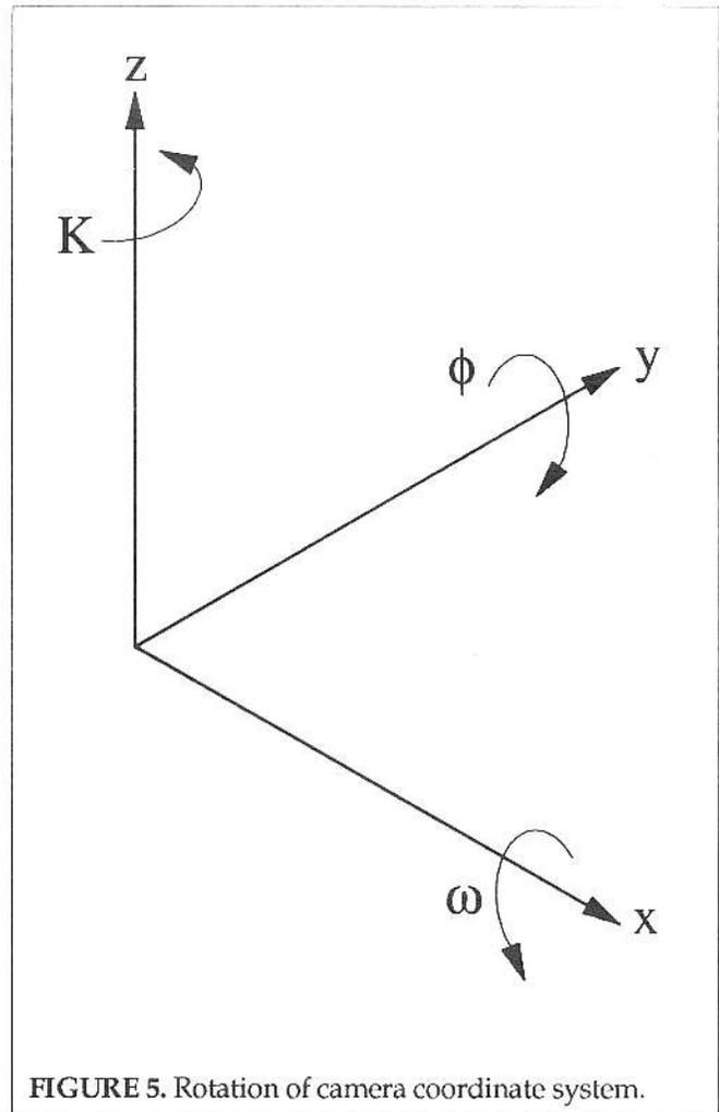
FIGURE 5. Rotation of camera coordinate system.
