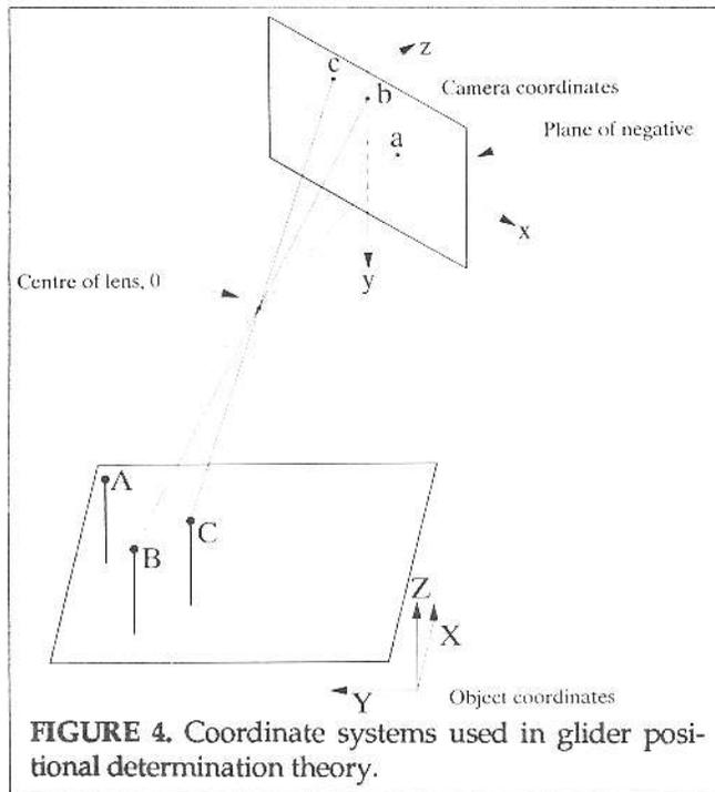
FIGURE 4. Coordinate systems used in glider positional determination theory.
