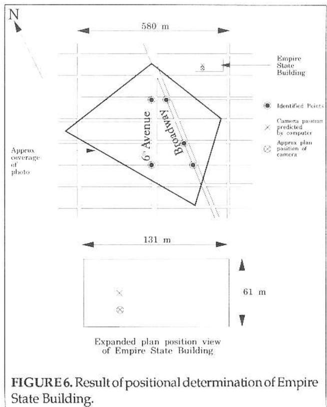
FIGURE 6. Result of positional determination of Empire State Building.
