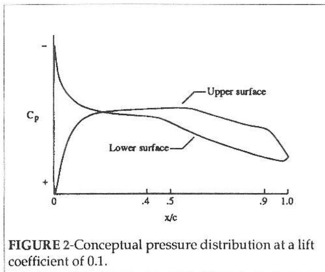
FIGURE 2-Conceptual pressure distribution at a lift coefficient of 0.1.
