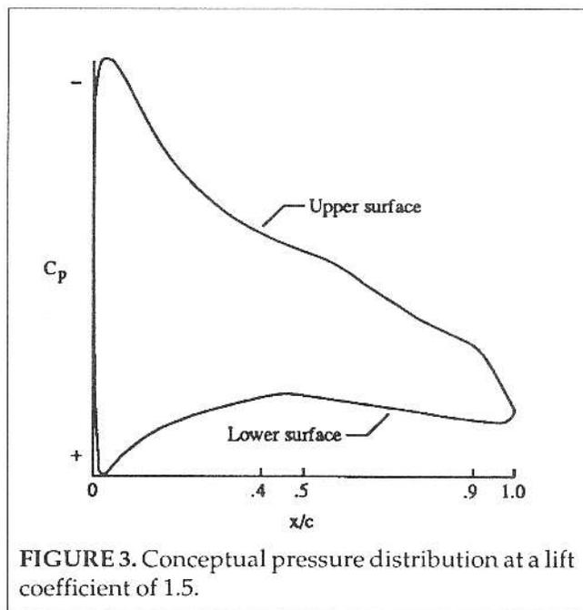
FIGURE 3. Conceptual pressure distribution at a lift coefficient of 1.5.
