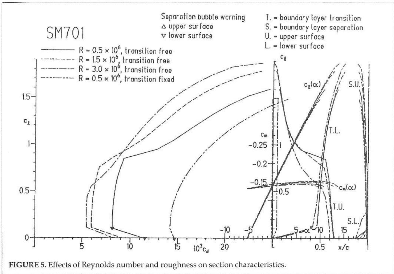
FIGURE 5. Effects of Reynolds number and roughness on section characteristics.
