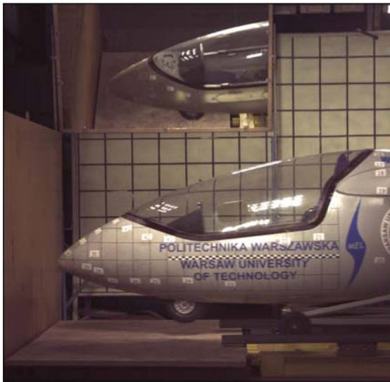
Figure 3 Experimental stand arrangement (the second test).
