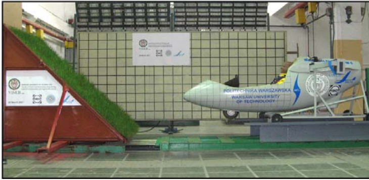
Figure 2 Experimental stand arrangement (the first test).
