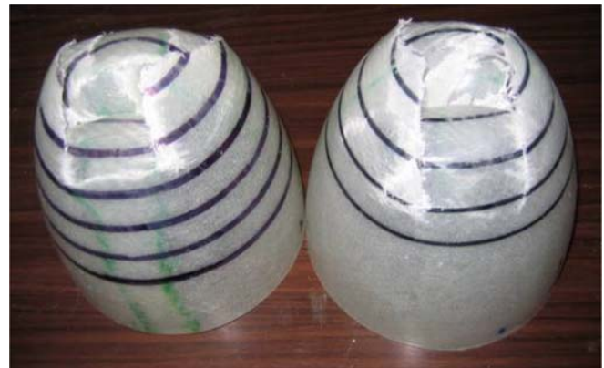
Figure 13 Specimens after impact.
