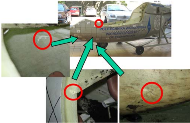
Figure 9 Small cracks observed after the first crash test.
