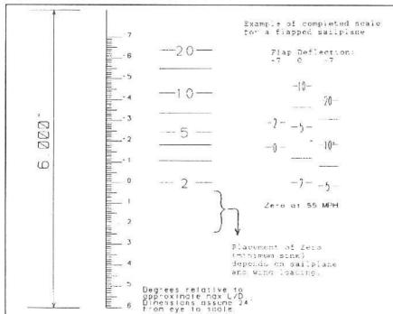
FIGURE 9. Implementation of pitch-to-fly scale. The pilot sights through this scale to the horizon to compare pitch attitude to the pitch-to-fly.
