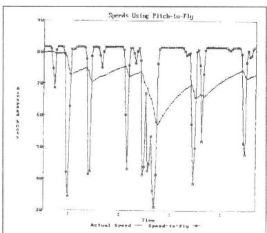
FIGURE 8. Pitch-to-fly airspeed vs. speed-to-fly for ASW-24. The airspeed obtained using pitch-to-fly is contrasted with the ideal speed-to-fly, especially during periods of acceleration.
