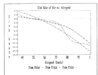
**FIGURE 5.** ASW-24. The sailplane polar was taken from the published calculations of the designer. Note the prominent transition from laminar to turbulent flow and its effect on speed-to-fly.
