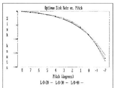
FIGURE3. Pitch-To-Fly versus L/D for a maximum L/D speed of 50 knots. Variometer reading as a function of optimum pitch attitude is essentially independent of sailplane L/D.
