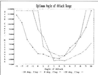
FIGURE 7. Drag coefficient as a function of angle of attack for several flap deflections of the UAG 88-143/20 airfoil. The optimum angle of attack is the same for all flap deflections.
