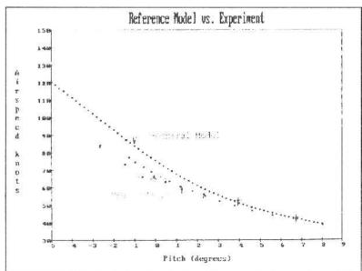
FIGURE 4. Blanik pitch attitude data. Measured airspeed vs. pitch attitude for a Blanik L-13 is compared to that predicted from the general analytic model and that predicted from the published polar.
