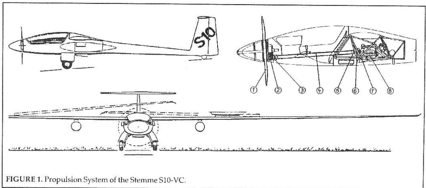
FIGURE 1. Propulsion System of the Stemme S10-VC.
