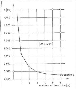
FIGURE 4. The optimization weight history for fuselage substructure.
