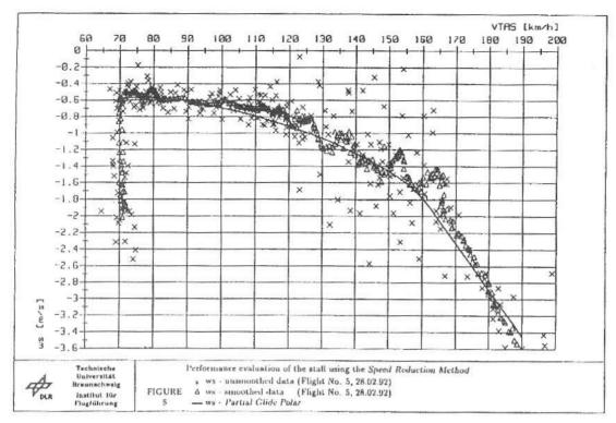
global rate of sink is the main reason for this difference. Therefore it is obvious that the measurements for a polar using the Speed Reduction Method should be done on different days. After eight experiments slight changes should still be expected, and the error of the Speed Reduction Method is approximately 8%, which is similar to the error of the Partial Glide Method.
