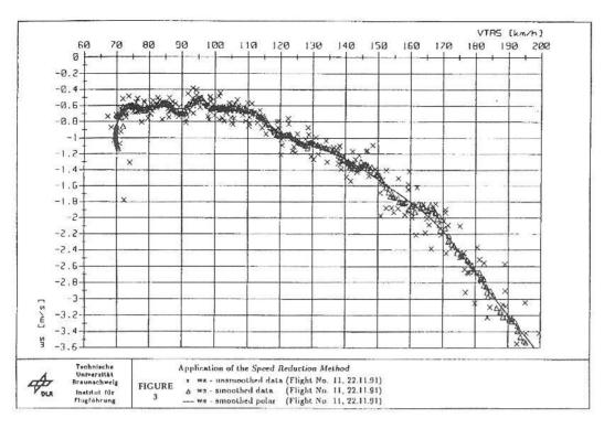
be reproduced. The Speed Reduction Method uses a horizontal flight path, which is indicated by the VP3-IMA. The speed at the beginning of the experiment is approximately 250 km/h. The advantage to prior tests close to ground is the speed reduction till stall speed. The investigation by Ortgies [3] showed that the stick movement should be restlicted to one way. If the horizontal flight path is left upwards, the pilot should not move tlle sticl;
