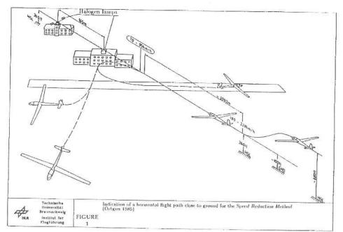
The basic idea of the Speed Reduction Method is the assumption that the lift and drag coefficients calculated from the instationary measured data are equivalent to those corresponding to the stationary airspeeds and rates of sink. Thus the equations for the stationary airspeed and rate of sink are expressed in terms of the lift and drag coefficient.
