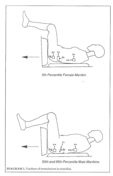
sitting upright for the actual test. The readings from the load cells give the actual load that would be experienced by a pilot, have been given in pounds force (lb. ft..) and in kiloNewtons (kN) in Table 2.
