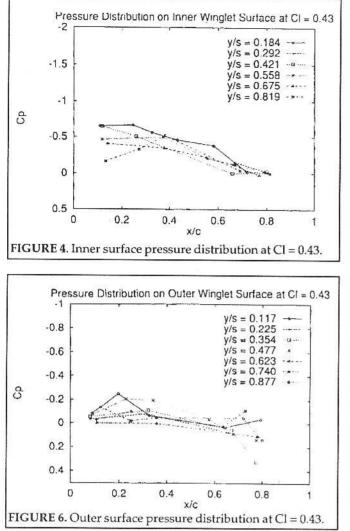
obtain more accurate CFD results it will be necessary to use a method that solves the entire flowfield near the winglet, probably an Euler code, which demands computational resources that are significantly more powerful than are necessary for a panel method. Pressure distributions are also shown for both the inner winglet surface and outer winglet surface at lift coefficients 0.43 and 0.6 in Figures 4, 5, 6 and 7.
