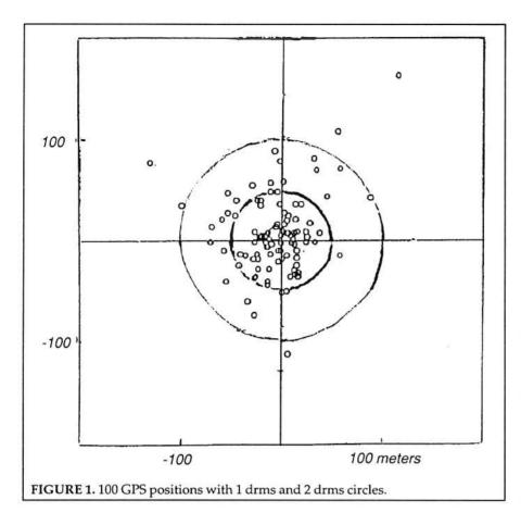
accuracy of 115 yards (1 drms). However, this figure does not take account of errors due to poor satellite geometry and weak signal strength. To cope with this particular problem the Garmin 55 calculates an estimated position error, based mainly on these two factors, and ceases to give a position if it exceeds 550 yards.
