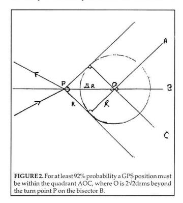
entire aircraft is proved to have been above the observation zone. This requirement of proof is the heart of the problem with GPS turn point verification. Whilst a turn point photograph can prove whether or not the entire aircraft was above the observation zone, a GPS measurement cannot. This is because, although it is remarkably good as a navigation aid, its absolute accuracy is always uncertain, unlike that of either a photographic or a geodetic measurement.
