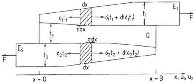
Figure 2. Sketch of the forces in a glued joint
