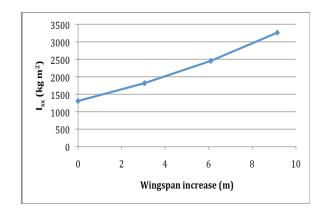
Figure 5 SGS 1-36 Estimated mass MoI variation with wingspan.
