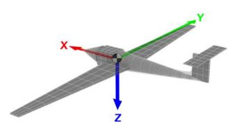
**Figure 2** Concept drawing showing the representation of sailplane components by geometric figures.
