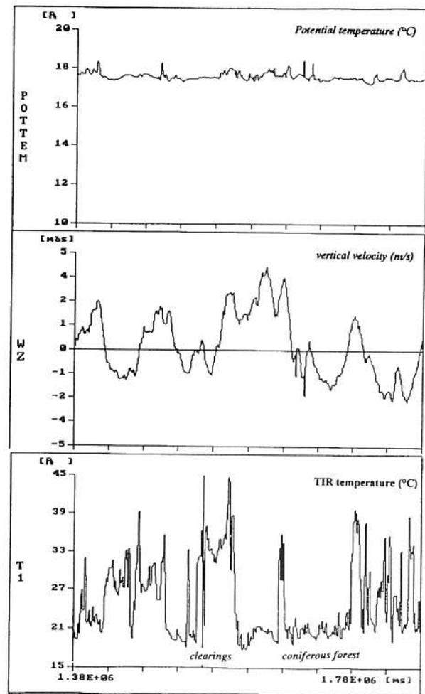
Figure 8. Quasi-horizontal flight legs over different kinds of soil and vegetation for vertical flux of sensible heat near Belzig, Germany on 17th of June, 1997 at 160 m GND.
