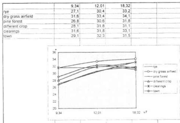
Figure 5. TIR temperatures ( $^{\circ}\text{C}$ ) of different surfaces at the 29th of June, 1997 at three different times: 9.34, 12.01 and 18.32 local time near Belzig, Brandenburg flight altitude between 200 and 300 m GND.
