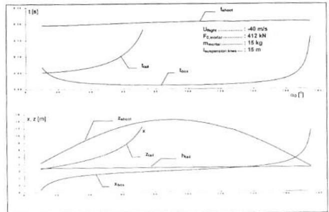
Figure 9. Characteristic values of the trajectory depending on the firing direction. Mortar deployment.
