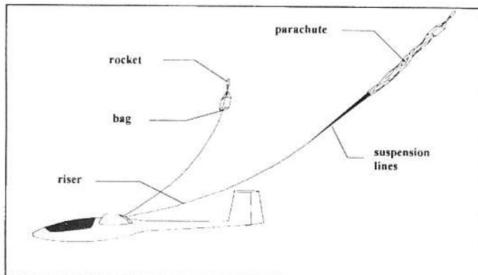
Figure 1. Rocket deployment, packed parachute.
