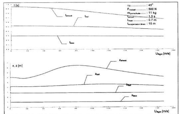
Figure 6. Characteristics values of the trajectory depending on flight velocity. Rocket deployment/packed parachute.
