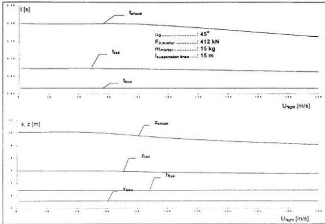
Figure 10. Characteristic values of the trajectory depending on the flight velocity. Mortar Deployment.
