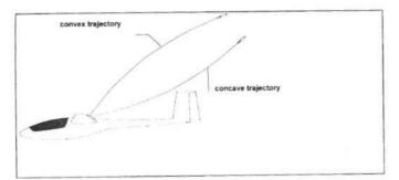
Figure 7. Convex/Concave trajectory.
