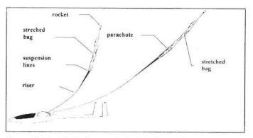
Figure 2. Rocket deployment, stretched parachute.
