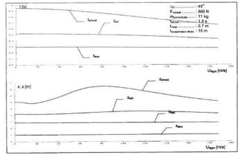
**Figure 6.** Characteristics values of the trajectory depending on flight velocity. Rocket deployment/packed parachute.
