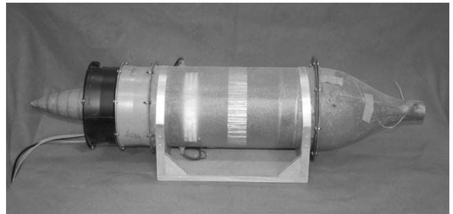
**Figure 7** Small free-stream wind tunnel of TU Berlin.
