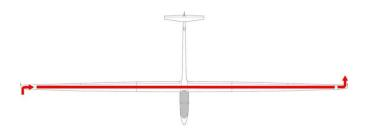
**Figure 2** Path of air flow through a complete span covered internal flow system in a typical high-performance sailplane.
