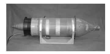
Figure 7 Small free-stream wind tunnel of TU Berlin.
