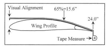
Figure 1. Measuring the Wing Chord.
