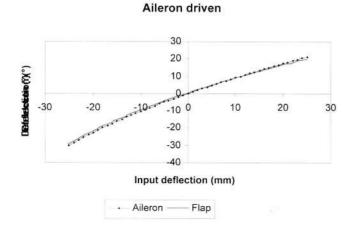
Figure 10: Aileron and flap deflection against input aileron deflection
