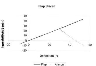
Figure 11 Aileron and flap deflection against flap input deflection
