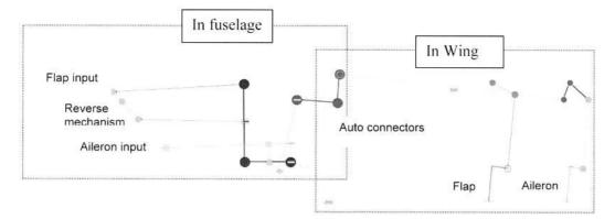
Figure 7:Excel representation of the Aileron flap mixer.
