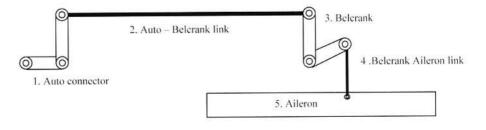
Figure 5: Aileron control system in aircraft wing
