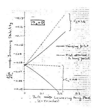
Figure A4,1 Stability versus hang point vertical location for a flying wing.
