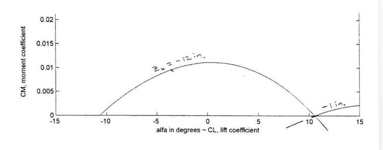
Figure A4,4 The effect of hang point vertical location on large disturbance stability.
