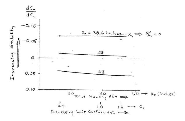
Figure A4,5 The effect of fore and aft position of the pilot and of the hang point.
