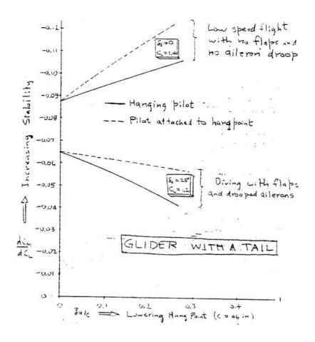
Figure A4,2 Stability versus hang point vertical location for a glider with a tail.
