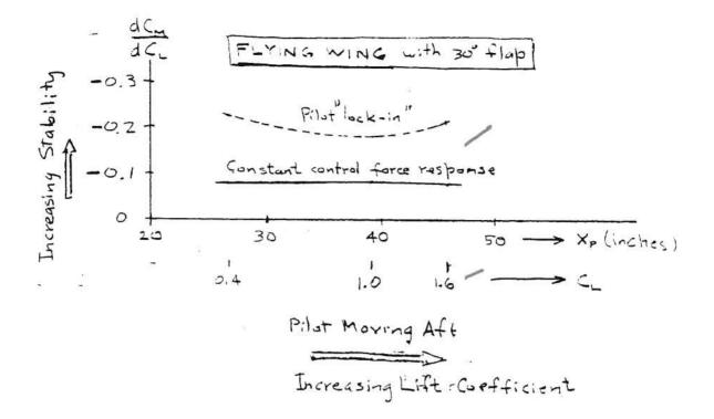
Figure A4,6 Comparison of stability for pilot "lock-in" and for constant-control-force pilot response.
