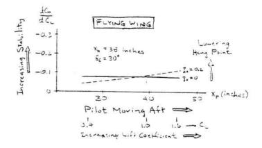
Figure A4,3 The effect of hang point vertical location on small disturbance stability.
