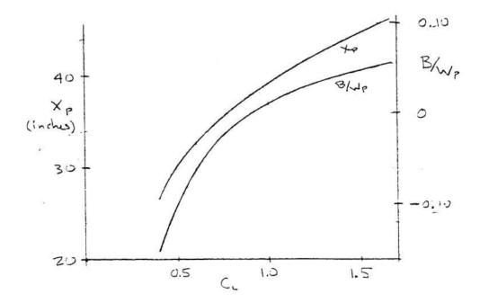
Figure A4,7 Pilot position and control force versus lift coefficient.
