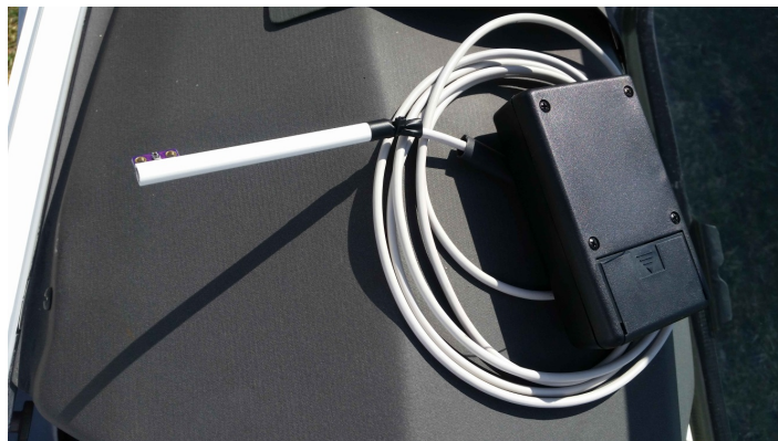
Fig. 2: Measurement hardware installed on the Ventus-2 glider.
