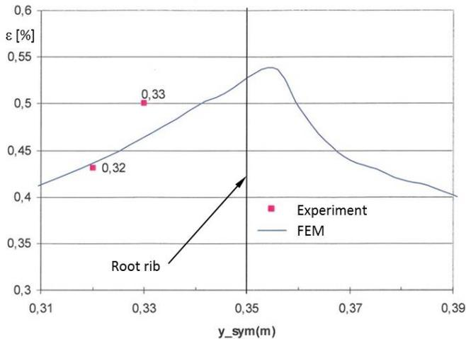
**Fig. 9: PIK-20D upper spar cap strains computed at limit load  $n=6,62$  and maximum weight  $m=450$  kg with a FEM model (FEM) and measured in the static test (Experiment). The numbers indicate the strain gage location from the symmetry axis, Lukkarinen [13] (page 70).**
