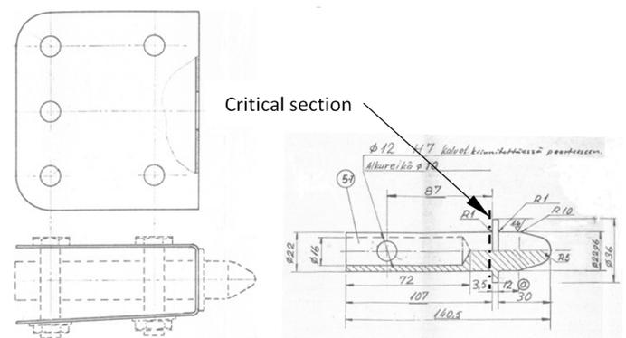
**Fig. 12: PIK-20D Wing spar end main fitting bracket.**
