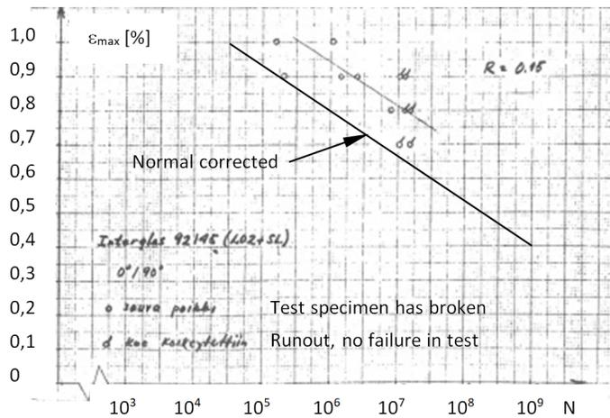
**Fig. 11: S-N curve of 0°/90° symmetric glass fiber laminate with Interglas 92145 cloth and Rütapox L02/SL resin system. The test was performed using a tension test coupon. The stress ratio has a value  $R = 0,15$  and  $\epsilon_{max}$  is the maximum strain in the cycle in the coupon 0° direction, Soinne [17] (page 27).**
