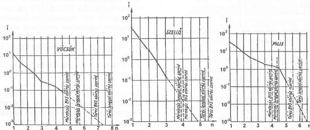
Figure 1. Landing Load Statistics for Three Types (Gedeon (10))
