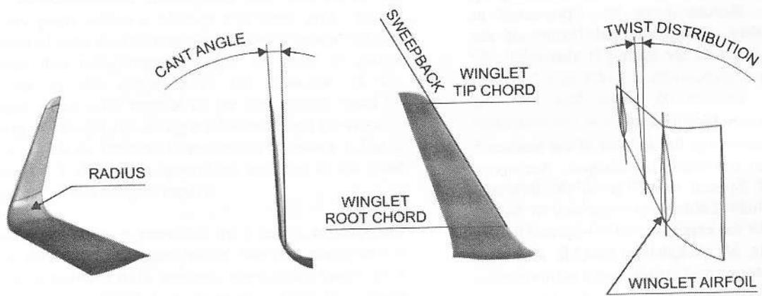
Figure 3. Key Parameters of Winglets
