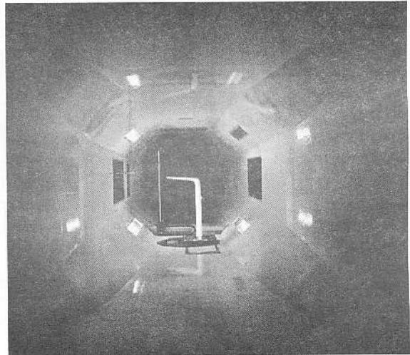
**Figure 7.** Winglet Models (1:1) Placed in Handley Page Wind Tunnel
