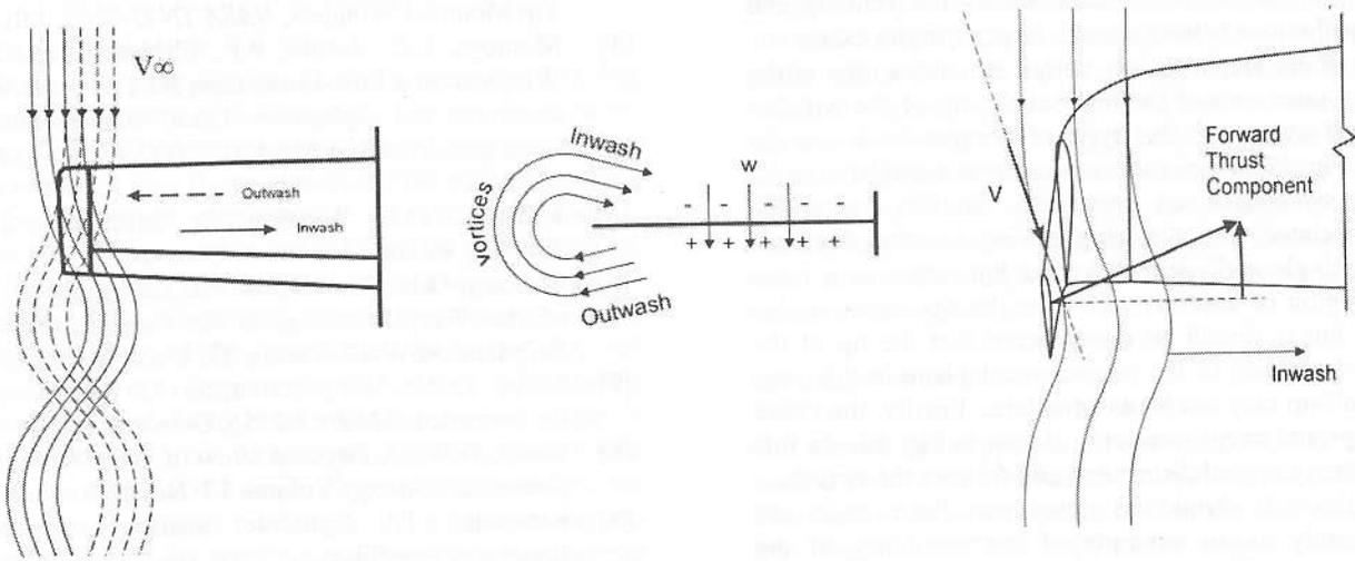
Figure 2. Forward Thrust Component Development
