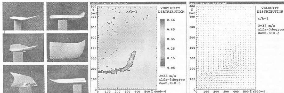
Figure 14. HpH 304 sailplane's wing tip for span of 17.43 meter - model D
