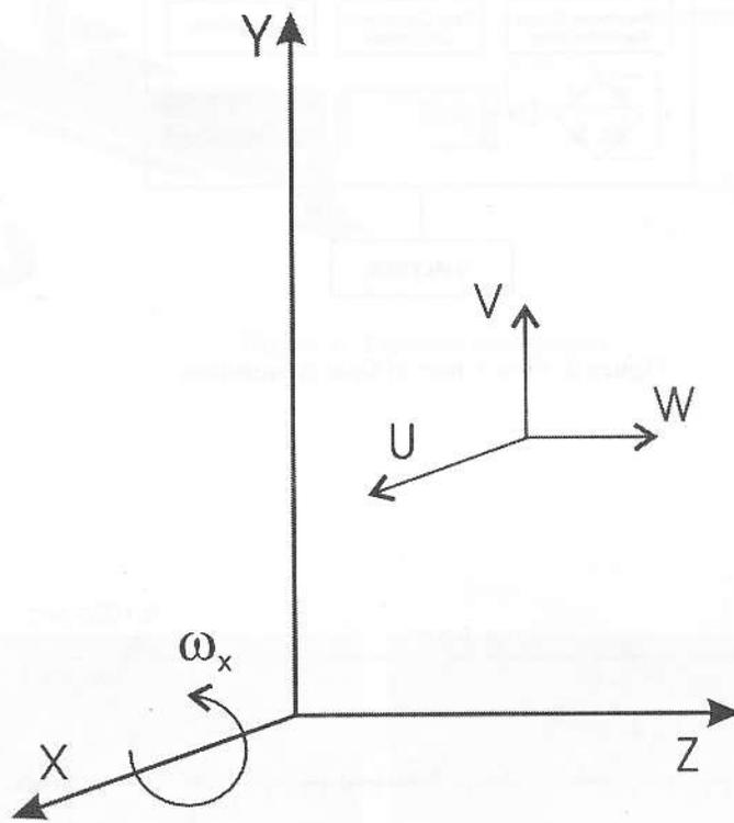
**Figure 10.** Coordinate system and velocity components definition
