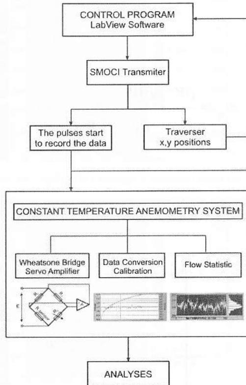
Figure 8. Flow Chart of Data Acquisition
