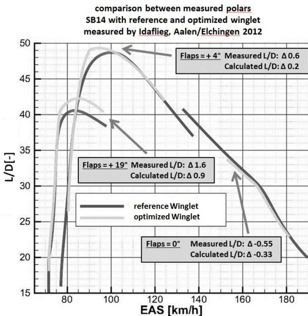
Fig. 12: Comparison of measured and calculated glider performance expressed by the glide ratio  $L/D$  versus airspeed.
