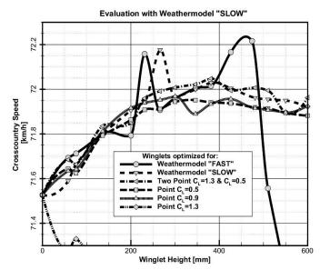
Fig. 7: Cross-country speed for model "SLOW" of optimized winglets with varying height h.
