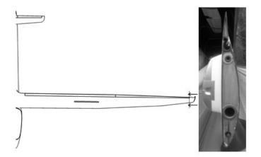
Fig. 2: SB 14 (and SB 15) wing-winglet connection.
