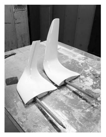
Fig. 11: Baseline SB 14 winglet (left), the reference for the performance flight tests conducted, and the optimized SB 15 winglet (right).
