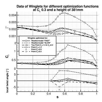
Fig. 10: Load distribution  $\Gamma$ , local lift coefficient  $c_l$  and twist angle variation  $\varepsilon$  vs. dimensionless true length *s*.
