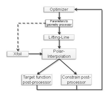
Fig. 1: Principle of the optimization process chain.
