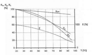
Figure 1. Influence of the temperature on mechanical properties of the epoxy composite reinforced by glass fabrics.
