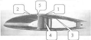
Figure 7. Cross-section of the wing and thermocouple sensors locations:
