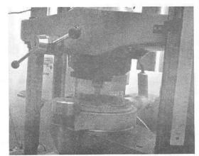
**Figure 3.** Tests of the wing spar material specimens performed on the strength machine at a temperature of 54 deg C.
