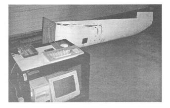
Figure 8. General view of the wing specimen and the system of temperature recording.
