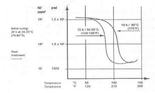
Figure 2. Change of G-modulus versus the temperature of epoxy resin L160 with the hardener 260S [2].
