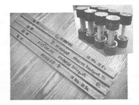
Figure 4. Specimens of composite used for examination of the glider spar flange manufacturing process (witness-specimens) in a raw form and ready for the strength (compression) test, respectively.
