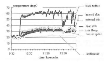
**Figure 13.** Diagrams of temperature measured in the wing structure during sunny day.
