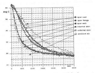
Figure 10. Cooling process of the PW-5 wing structure after heating in 62 deg C.
