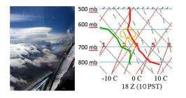
Fig. 14: Schematic of the process that produces rotor clouds in a stable, unsaturated environment. The yellow lines illustrate the cloud formation process.
