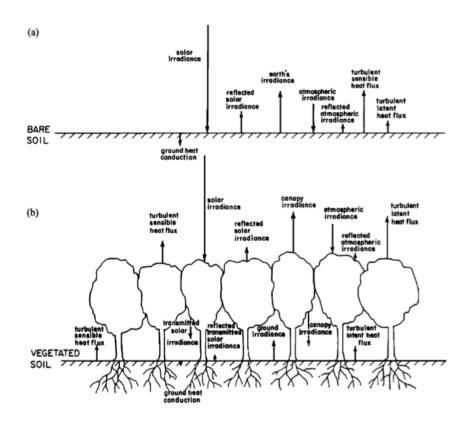
Fig. 1: Schematic illustration of the surface heat budget over (a) bare soil and (b) vegetated land [2].
