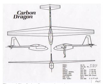
Figure 1 The Carbon Dragon schematic
