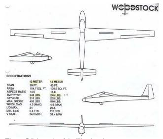
Figure 5 Schematic of the Woodstock
