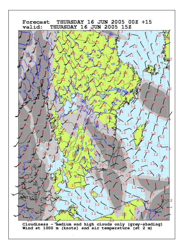
**Figure 2** A winds and temperature forecast chart. The amount of medium and high clouds as grey shading in the same way as in the thermal chart (notice, the low clouds are excluded). Temperature in the air near the ground (2 m) plotted with red figures (blue if below zero). Wind at approximately 1000 m plotted in the way it is usually done on weather charts, wind arrows with barbs (a full barb means 10 kts and a half barb 5 kts. For strong winds a streamer means 50 kts.)
